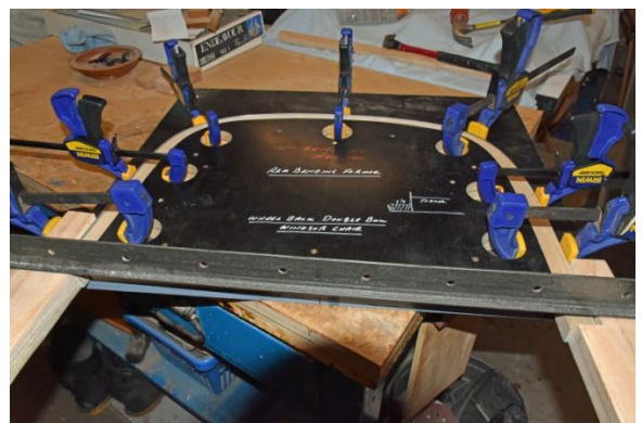
Figure 4 view of the bent arm, look closely and you can see how the compression band holds the wood in compression whilst it is bent.
