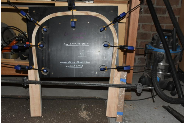
Figure 5 The bow in the bending former, waiting to completely dry before being removed.
