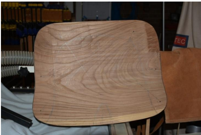
Figure 1 The seat cut and shaped with the holes marked for the legs and arm post.
