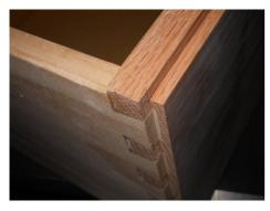
The method I use to fit Cock Beading to a drawer front, is to cut a rebate around the edge of the drawer face after I have made the drawer. This rebate is usually cut to accommodate Cock Beading 6mm thick by 10mm deep.
