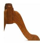
The wood grain in the legs of this pedestal table runs parallel to the longest dimension, making the legs as strong as possible. Were the grain to run parallel or perpendicular to the pedestal, the legs would be weakest at their narrowest point, the ankles.
