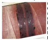
rendering it unusable. The cause of this is either attempting to take too great a cut or running the belt at too slow-a-speed. In oscillating mode, the drive belt MUST BE RUN AT MAXIMUM SPEED! As a
