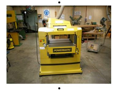
The thicknesser has been serviced, with all 150 cutters being individually cleaned and rotated. The table and rollers have been stripped back to the bare metal and recoated with Silber Glide. This service took almost nine man-hours to complete, and the machine is performing like new. I once again remind Members that the use of the metal detector is MANDATORY on all timber going through this machine. Even new timber can have staples present. Timber MUST BE VISUALLY CHECKED for foreign matter,
