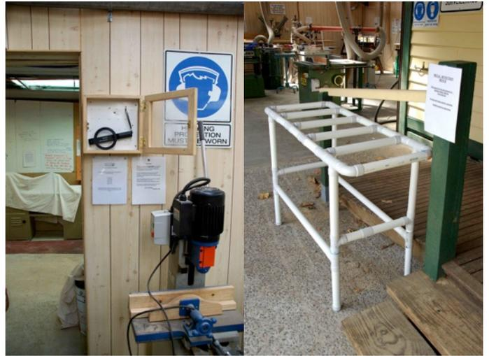
**2. Ensure that the dust extraction system is turned on!** The blast gate has been removed from the thicknesser, but we have since had an instance of someone using the machine with the extraction system turned off. This will jam the table rollers and probably ruin your project.
