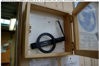
IS **ESSENTIAL THAT ALL** INCLUDING NEW, BE SCANNED **BEFORE** BEING PASSED THROUGH ANY OF THE CLUB'S MACHINES! TIMBER SHOULD ALSO BE INSPECTED FOR NON-METALLIC FOREIGN MATTER SUCH AS DIRT AND STONES, AND PAINT SHOULD BE REMOVED AT HOME. FAILURE TO DO THIS NOT ONLY LEADS TO THE **UNNECESSARY DESTRUCTION** EXPENSIVE BLADES, BUT CAN RUIN THE WORK OF THE NEXT MEMBER TO USE THAT **MACHINE!**
