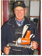
Here also is Peter Jordan with a jig he made to fit on his wood lathe to make drilling quicker, more accurate and reproducible.
