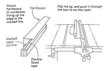
Here's a quick and foolproof way to cut tapers. First draw the desired cut line on the workpiece in pencil. Set the saw fence to a width slightly greater than the workpiece, and cut a scrap of hardboard to this width. Using either double-faced tape or tacks, affix the hardboard to the workpiece, carefully aligning the edge of the hardboard to the pencil line. Run this assembly through the saw without resetting the fence.
