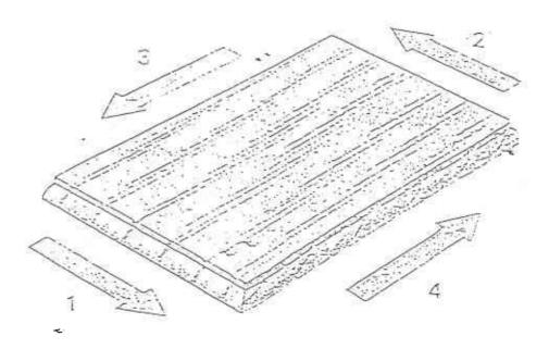
Avoiding tearout: Tearout generally occurs at the end of a cross-grain cut because the fibers at the end of the cut are not supported. If you rout across the grain first, tearout can be routed away with the long-grain cuts.
