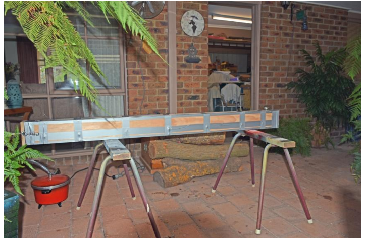
Figure 3 My steam box and steam generator, about to be tested.
