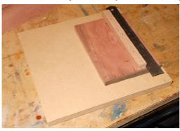
I use brass butt hinges and I want them flush at the back. Fitting the hinges to the box carcase is easy, but getting the lid to line up flush is not so easy. It is fiddly to line up. So I made up a jig using a lid made from some left over scrap. the jig is just a stepped stop.
