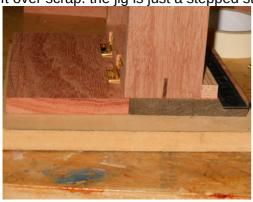
The box lies on the jig while the lid slides up to it, looking at the picture I have aligned the lid so it will be flush at the back. Everything can be clamped in place to enable you to drill your screw holes (I usually drill and screw one at a time so I can keep checking the alignment and fit)
