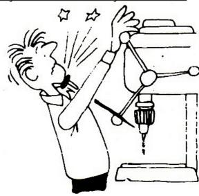
No 3. Remove adjusting keys and wrenches. Form a habit to check for keys and adjusting wrenches before turning any machine on.
