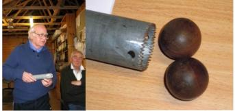
**Ray Easthope** showed us his ingenious, homemade ball-turning-tool, fabricated from a piece of pipe.
