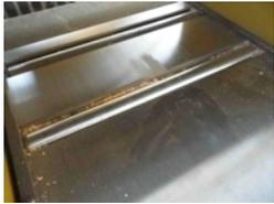
The two table rollers are prone to jamming due to chip buildup. Before using the machine, rotate the rollers by hand, and if they do not rotate freely, use compressed
