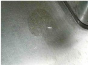
being dropped on it. The raised lip around the small dent would have produce scratching on the surface of any timber being passed over it if
