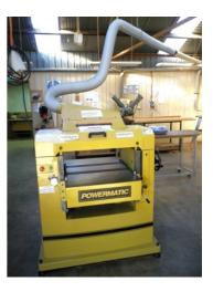
**3.** Ensure that the timber is free of dirt, stones, etc. If necessary brush or sand to remove contamination prior to putting timber through the thicknesser.
