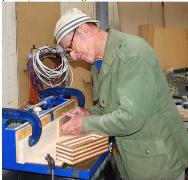
The box is on the router table made from layers of Merbau and Pine. It has a removable interior tray and will certainly look great when stained and felt-lined inside.
