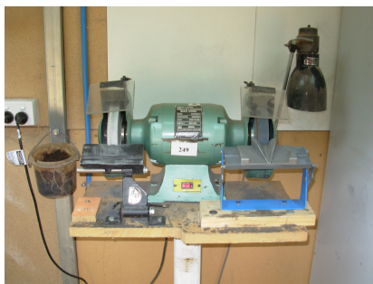
Double Ended Grinder Chisel Sharpening.
