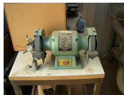
Double Ended Grinder Drill Sharpening.
